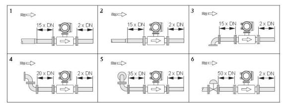
1 = Reduction, 2 = Expansion, 3 = 90° elbow or T-piece, 4 =  $2 \times 90^{\circ}$  elbow, 5 =  $2 \times 90^{\circ}$  elbow (3-dimensional), 6 = Control valve.
