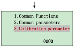
In this interface, press<sup>SET</sup> to enter the calibration parameter password input.
